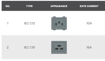
Note: The dimensions of GB10A / 16A outlets are different.
