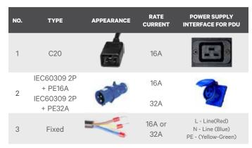
Note: The dimensions of IEC60309 2P + PE 16A / IEC60309 2P + PE 32A plugs are different
